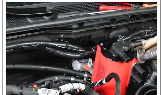
Install the AOS assembly onto the firewall studs.
