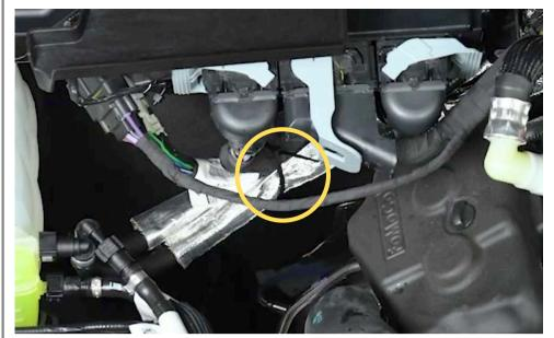
Slide the heat wrap back on the coolant hoses so that it protects the hoses from the back of the motor.
