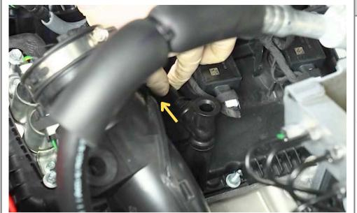
Install new Dipstick Adapter into dipstick tube.
