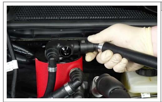
Prepare the 17" AOS Intake Pipe Hose, install 45° end onto AOS top port.
