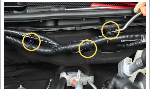
Using a small pry tool, loosen the wiring harness from the firewall by removing these three clips.
