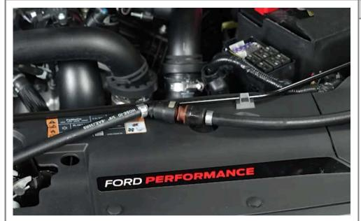
Install the 45° end of the Intake PCV Hose onto the PCV Valve.
