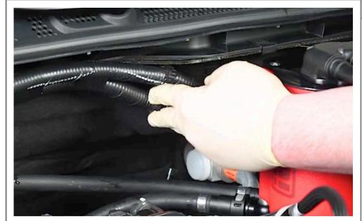
Reinstall the wiring harness clips onto the studs
