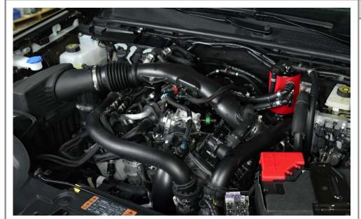
Reinstall the Upper Intake Pipe.
