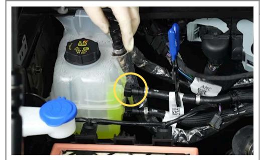
Disconnect the upper coolant reservoir hose, some coolant will escape.
