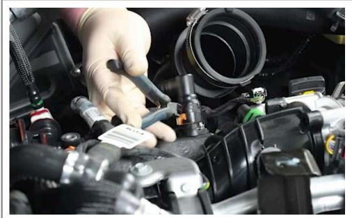
Locate the vent hose on the driver side valve cover.
