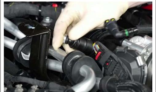
Install the 45° Intake PCV Hose end to the Intake Manifold.
