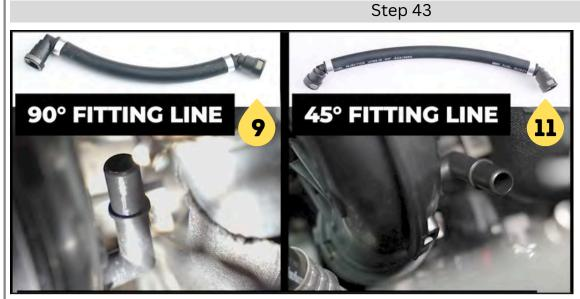
Determine intake pipe fitting style.
