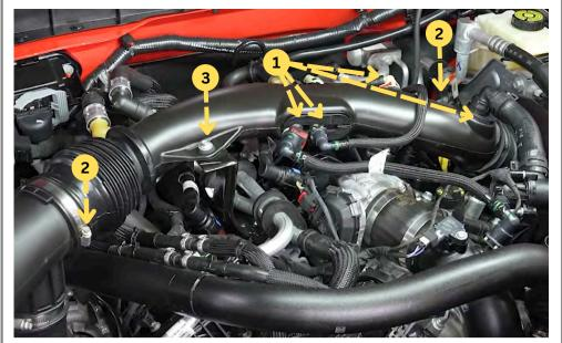
Remove the top intake pipe.
