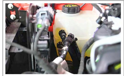
Connect the AOS coolant hoses inline to the coolant reservoir, and the factory coolant hose.
