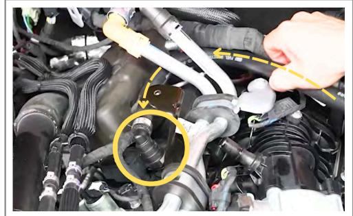
Install the opposing 90° end onto the passenger side valve cover port.
