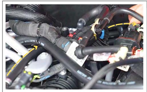
Route the AOS vent hose underneath the wiring harness and towards the back of the motor.
