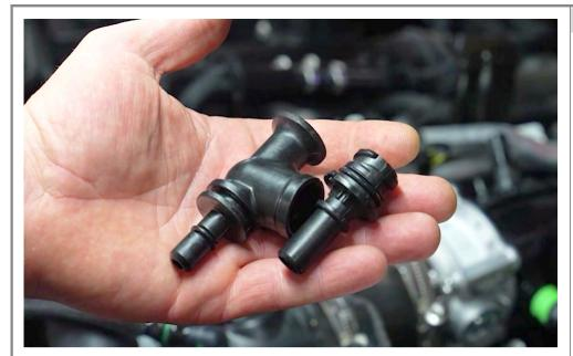
Prepare and assemble the new dipstick adapter and check valve.
