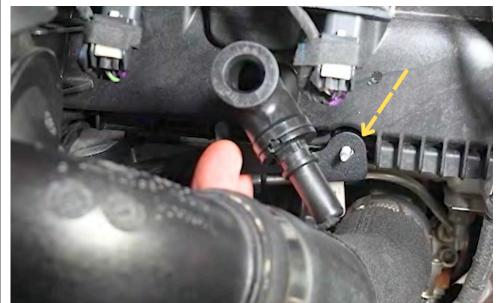
Install the dipstick tube bracket onto the stud. Ensure that the bracket is fully seated on the new dipstick tube adapter. Install a 8mm nut on the stud and tighten.
