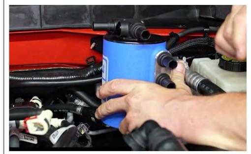
Position the AOS onto the firewall as shown.
