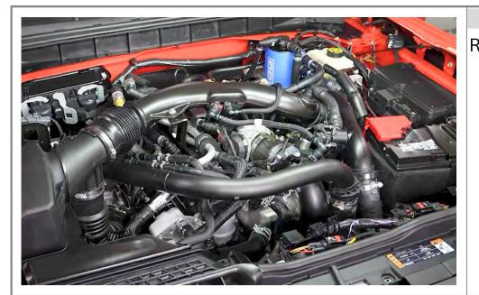
Step 46 Reinstall the top intake pipe.
