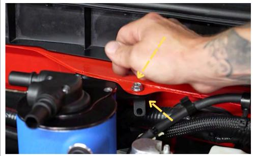
Install the provided 10mm bolt through the top of the AOS bracket, hand tighten the provided 10mm nut to the bottom of the bolt.
