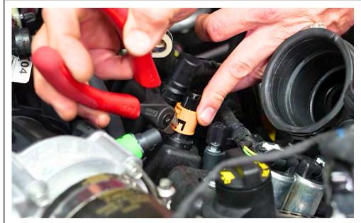
Remove the inner lock from the valve cover port.
