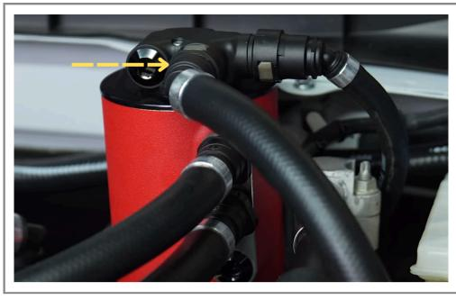
Install the 45 degree fitting from the 18" vacuum line to the top breather port on the AOS.
