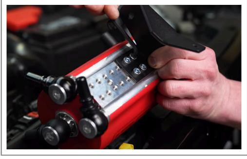
Install AOS bracket using 5mm allen bolts leaving five holes showing at the bottom.
