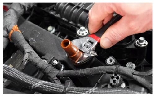
Step 2 Remove the OEM PCV fitting.
