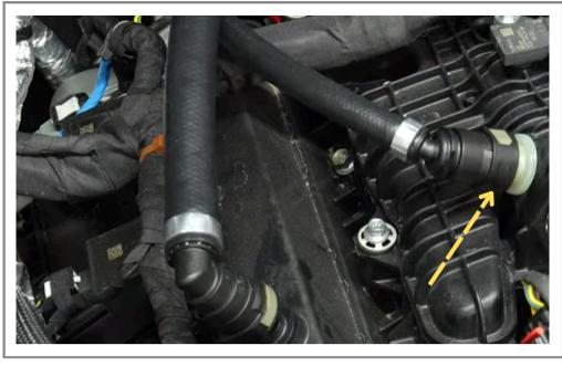
Install the PCV line with the two 45 degree fitting to the port on the intake manifold.
