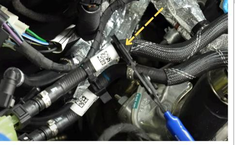
Clamp off the OEM coolant line at the top of the coolant reservoir.
