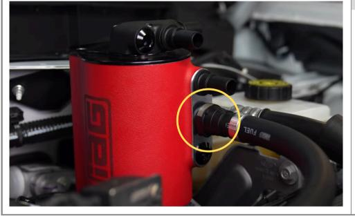
Install the PCV line onto the lower side port of the AOS.
