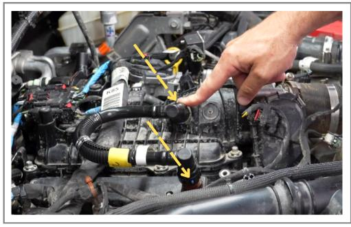
Remove passenger side PCV line. Push on the blue tab to lift off.
