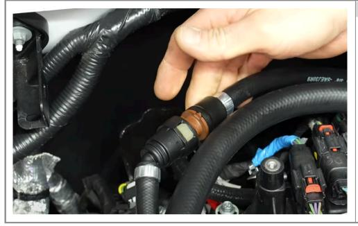
Install the OEM PCV valve to the PCV line.
