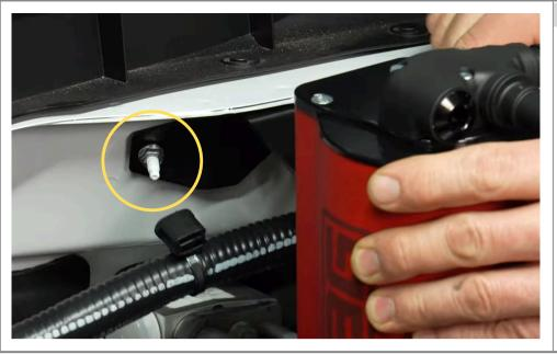
Install the AOS by screwing a 10mm nut onto the stud.
