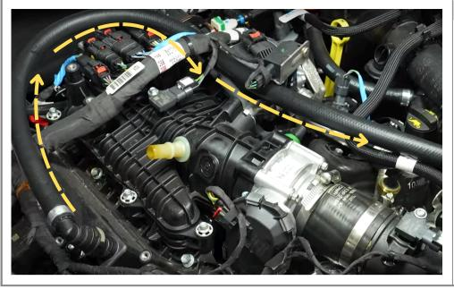
Route the PCV line under the wiring harness and bracket and towards the AOS.
