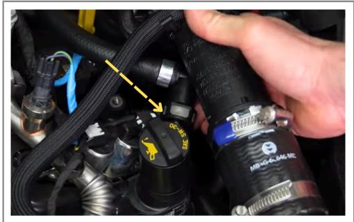
Step 24 Install the 90 degree fitting onto the oil filler neck drain port.
