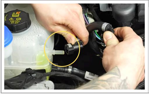
Connect the other coolant line to the coolant reservoir.
