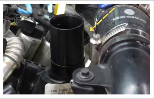
Install the new oil filler neck first. Twist clockwise to install.
