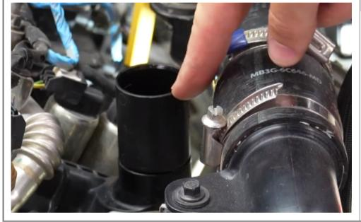
Remove oil filler neck by turning counterclockwise (if equipped).
