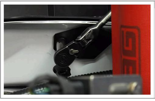
Tighten the 10mm nut to the stud on the other side using a 10mm socket.
