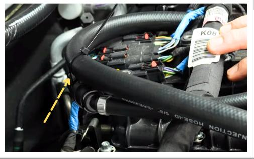
Install a zip tie to hold the lines together. Cut excess zip tie.
