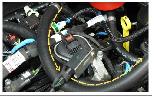
Route the driver side PCV line on top of wiring harness and under the wiring bracket.
