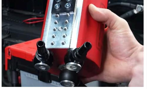
Rotate the coolant fittings to the back of the AOS.
