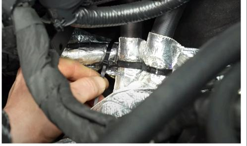
Zip tie the two coolant lines to the wiring harness located under the powertrain coolant module.
