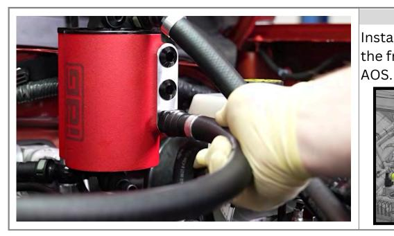
Step 29 Install the opposing end onto the front facing port of the
