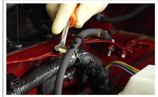
Using a pry tool, remove the ground cable fastener from the firewall.
