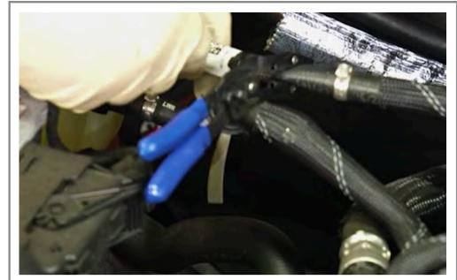
Using pinch off pliers, apply pliers to upper coolant reservoir hose.
