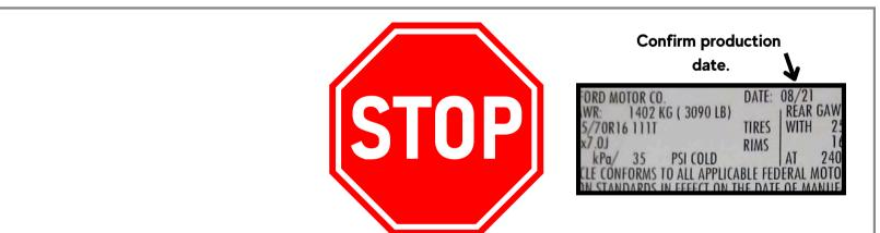
Please check the production date of your vehicle to confirm the correct fitment of the kit. This can be found by checking the vin plate in the drivers door well.
