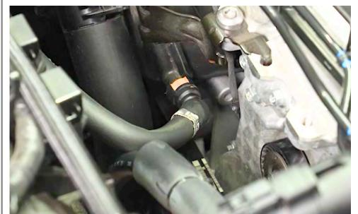
Following the same process, Remove the opposing end of the hose from the intake pipe.
