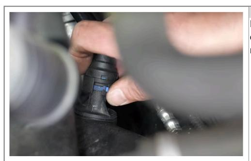
Step 12 Push on the blue tab for the other end of PCV line and remove from the inlet pipe.
