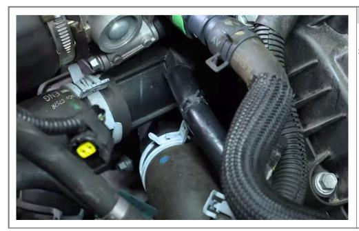
Step 32 Install the new coolant line from step 21.
