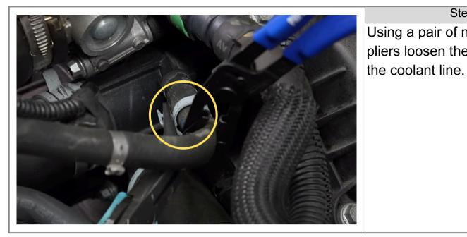
Step 30 Using a pair of needle nose pliers loosen the clamp from
