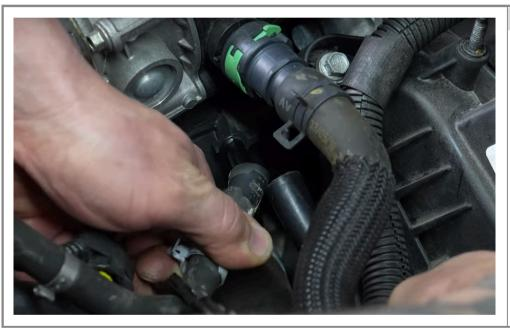
Step 31 Remove the OEM coolant line.
