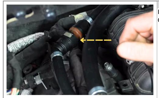
Step 47 Install the other fitting to the OEM PCV valve from step 44.
