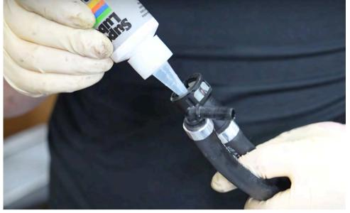
When installing the quick disconnect fittings, it is recommended to apply a small amount of multipurpose automotive grease/lube to the O-rings.
