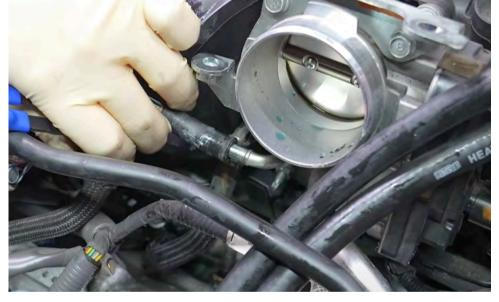
Remove the coolant line from the throttle body.
