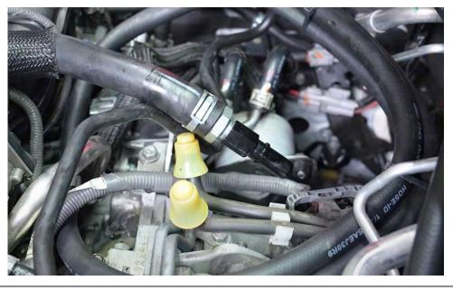
Install the PCV valve onto the factory intake manifold hose.
