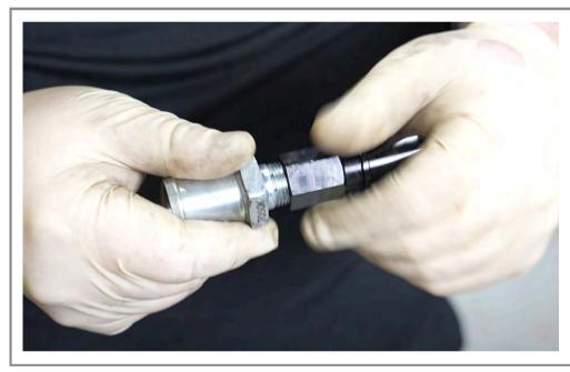
Step 39 Thread the PCV valve onto the PCV adapter fitting.
