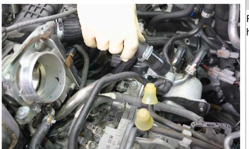
Step 13 pt. 2 Remove the intake manifold hose from the PCV valve.
