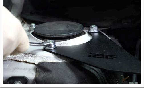
Reinstall the strut tower nuts and tighten.
