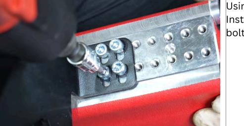
Using a 5mm Allen wrench, Install and tighten the AOS bolts.
