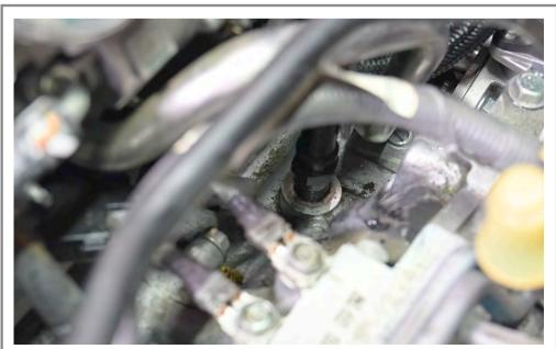
Step 16 Install the PCV adapter fitting into the block with a 19mm socket.
