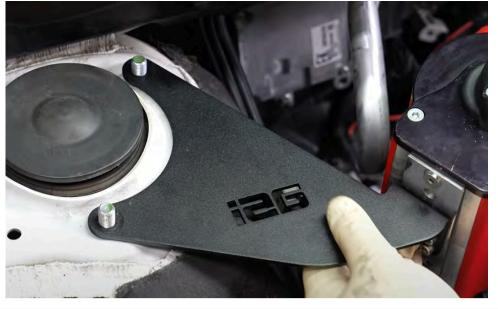
Install AOS assembly onto the strut tower.
