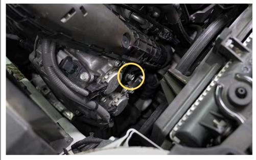
Remove the 12mm bolt from the charge pipe.
