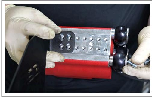
Assemble the AOS unit and bracket. Position the AOS bracket as shown, leaving 5 holes open toward the bottom.
