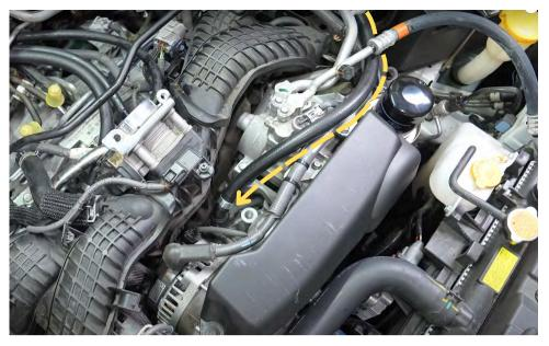
Route the hose underneath the factory A/C line as shown and connect the fitting onto the factory vent port.
