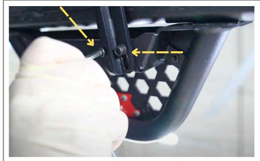
Prepare the step mounting hardware. Assemble the washers onto the 5mm Allen bolts.
