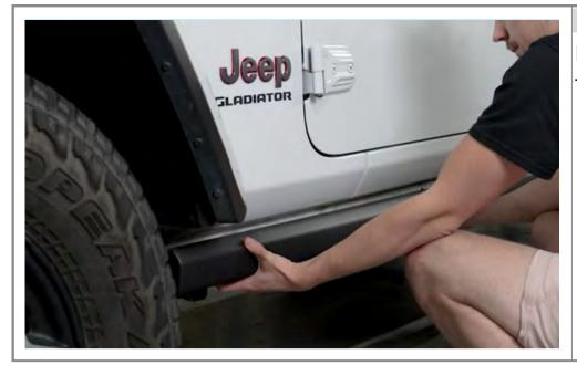
Remove the rock rail from the vehicle.
