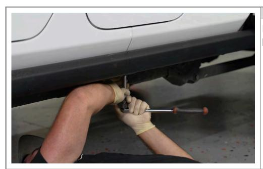
Step 8 Reinstall the rock rail hardware.
