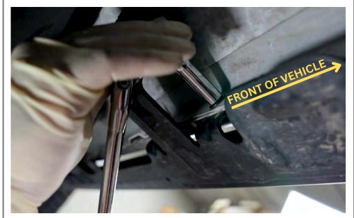
Locate the rock rail bracket underneath the drivers door.
