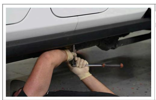
Step 5 pt. 2 Reinstall the rock rail hardware.
