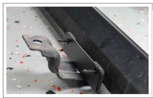
Step 4 pt. 2 Install spacers onto the remaining bracket.
