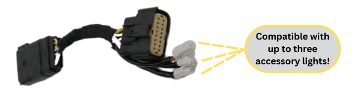
The Headlight Adapter Harness comes with three small electrical connectors. These are provisions for additional lighting equipment and may not be used.
