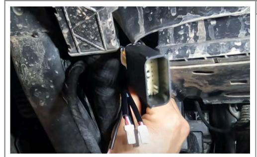
Install the provided Headlight Adapter Harness onto the headlight.
