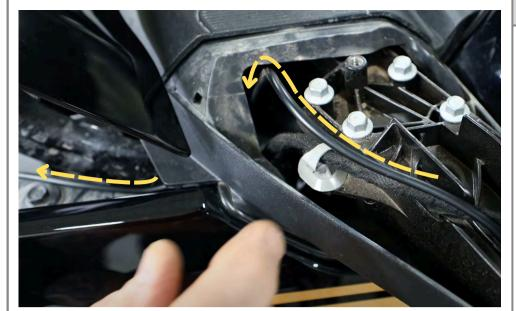
Route the wiring harness underneath the cowl, and into the engine bay as shown.
