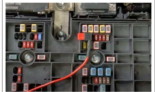
Install the fused wire end into the fuse slot.
