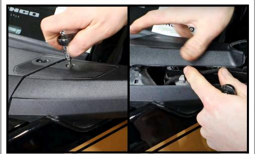
Using a Torx 25 socket, remove the bolt from the top mirror cover.
