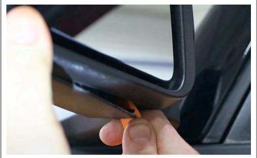
Using the provided pry tool, insert the tool into the bottom corner of the mirror cap. Carefully pry the cap away from the mirror.
