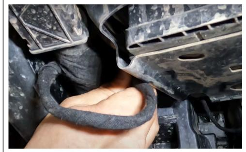
Partially remove the fender liner.
