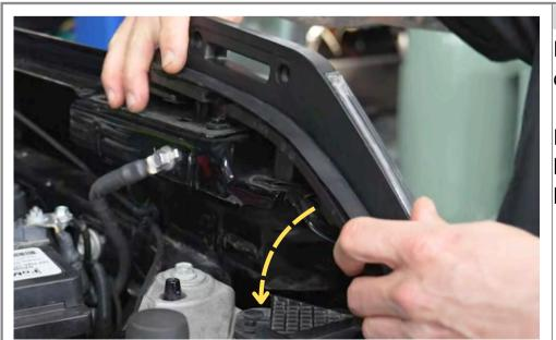
Step 7 Install new Trail Marker Light onto vehicle.
