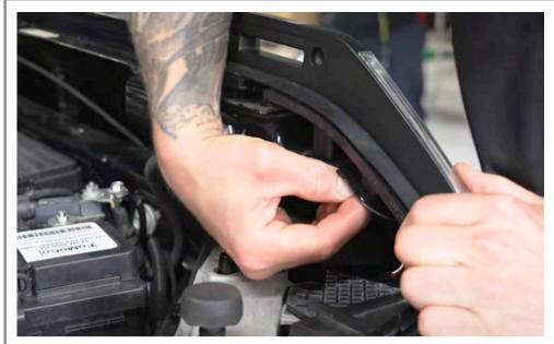
Install two provided 10mm bolts into the bottom of the Trail Marker Light.
