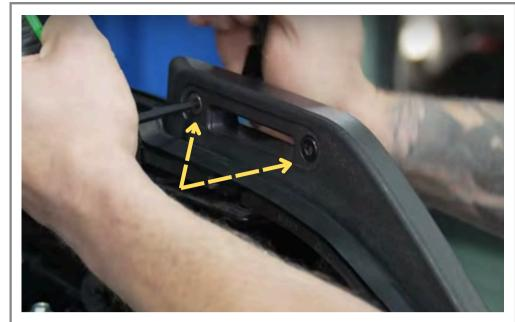
Remove the two TORX 30 bolts and nuts from the driver side factory Trail Marker.
