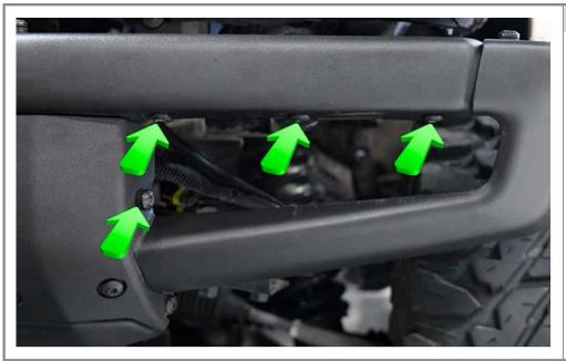
Remove the four TP40 Bolts from the drivers side of the front bumper.
