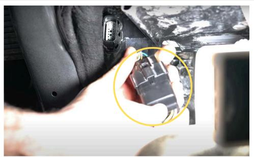
Step 5 Install the provided wiring harness adapter into headlight connector.
