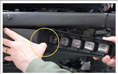
Step 2 Install the new Indicator. Carefully pry back the trim on the inner part of the bumper, and insert the Indicator behind trim.
