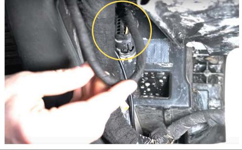
Remove some of the fender liner clips and fold back fender liner. Locate the headlight connector on the back of the headlight. Unplug the connector.
