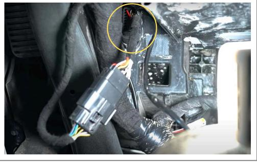
Install the wiring harness adapter into headlight socket.
