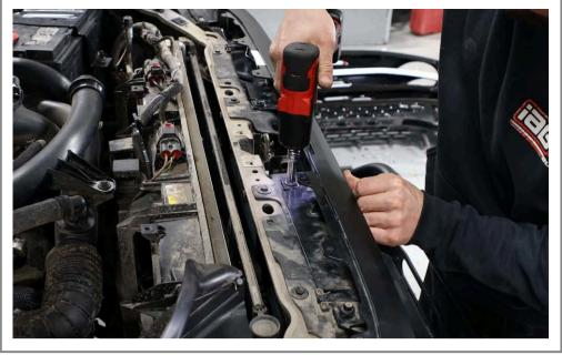
Reinstall and tighten the four 10mm bolts for the grille.
