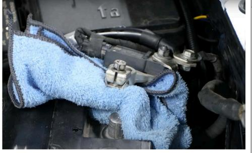
Disconnect the negative terminal of the battery.
