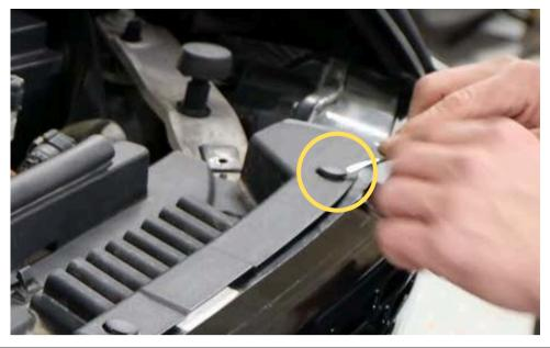
Using a small pry tool, remove the nine push clips from the radiator shroud.
