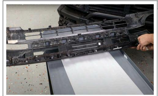
Reinstall the grille bracket, and tighten the six screws.
