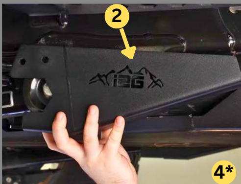
Step 6: Install the Passenger Side Skid Plate onto the lower rear trailing arm. (Spacers may be required depending on fuel tank skid)
