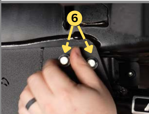
Step 4: Install two 12mm bolts through the outside of the Skid into the Bracket. Tighten all three 12mm bolts. (34Nm)
