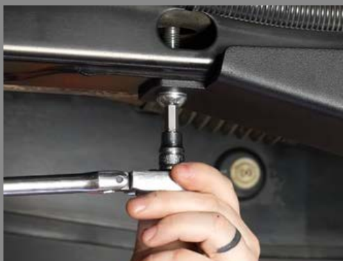
Step 5: Tighten the 8mm Allen bolt. (100Nm)
