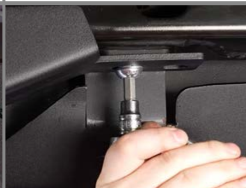
Step 10: Tighten the 8mm Allen bolt. (100Nm)
