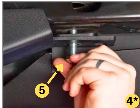
Step 7: Install the 8mm Allen Bolt with Washer into the Skid, do not tighten. (Spacers may be required depending on fuel tank skid)
