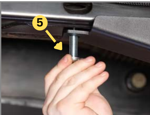
Step 2: Install the 8mm Allen Bolt with Washer into the Skid, do not tighten.
