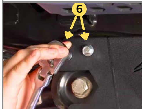
Step 9: Install two 12mm bolts through the outside of the Skid into the Bracket. Tighten all three 12mm bolts. (34Nm)
