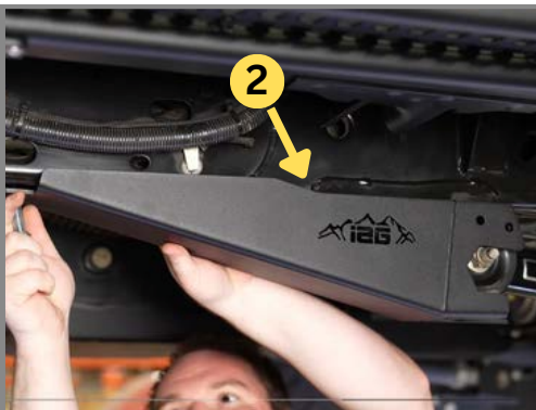
Step 1: Install the Driver Side Skid Plate onto the lower rear trailing arm.
