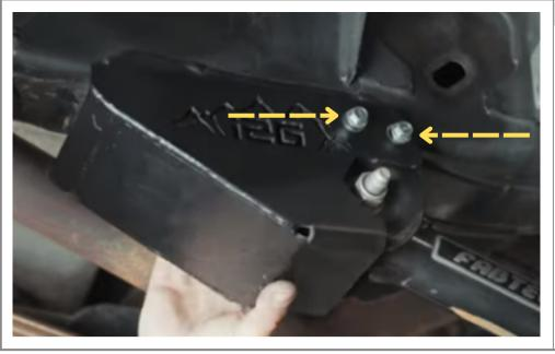
Install two 12mm bolts to the **outer** side of the skid plate.
