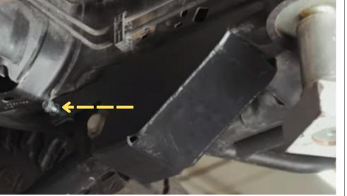
Note: Do not tighten the 12mm bolt.
