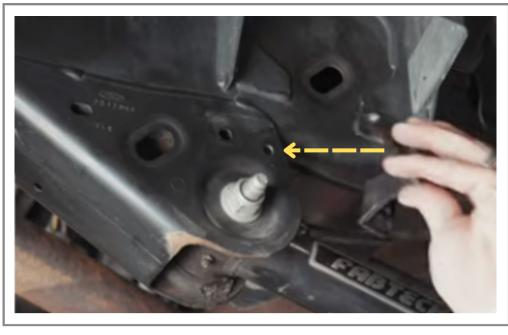
On the drivers side install the trailing arm bracket by sliding it in from behind the trailing arm.
