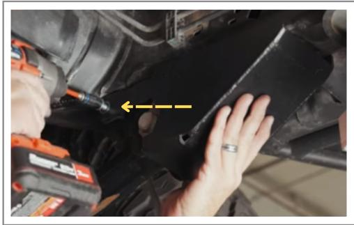
Step 6 Tighten the 12mm bolt on the inner side of the skid plate.
