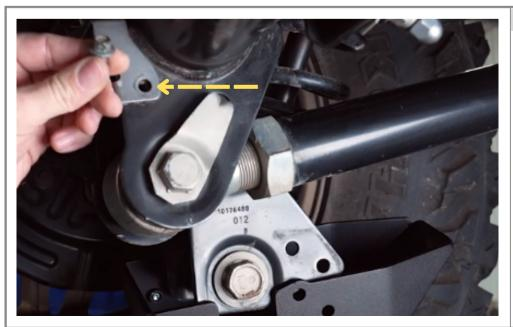
Step 9 Remove the 10mm brake line bracket bolt.
