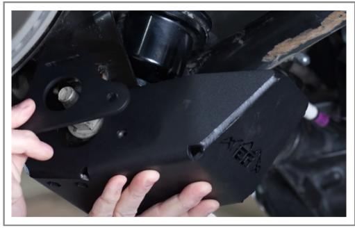
On passenger side install the passenger shock skid plate and one outer bracket.
