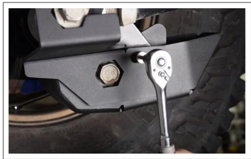
Step 12 Tighten the inner 5mm allen bolts on both driver and passenger sides.
