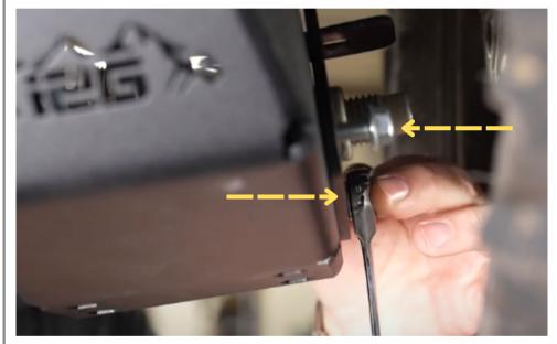
Step 14 Tighten the outer 12mm bolts on both driver and passenger sides.
