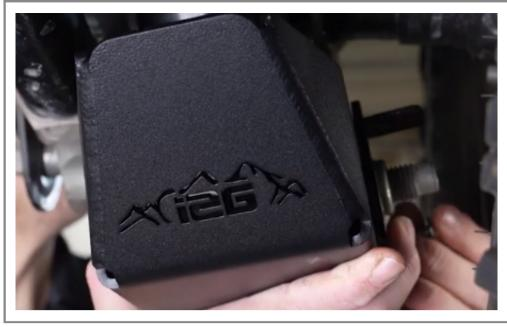
On driver side install the driver side shock skid plate and outer bracket.
