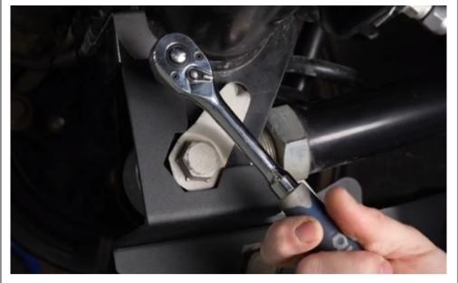
Tighten the 10mm brake line bolt.
