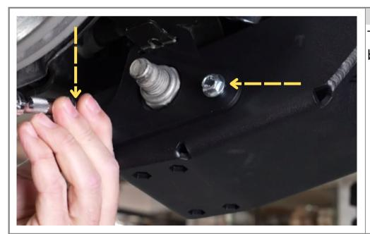
Step 6 Tighten the outer bracket bolts.
