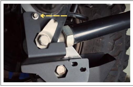
Install the inner driver side bracket using the factory brake line bracket 10mm bolt.
