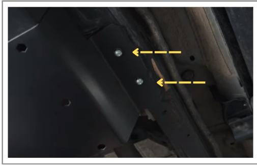
Step 5 Install two 6mm allen bolts and washers into each of the clip nuts.
