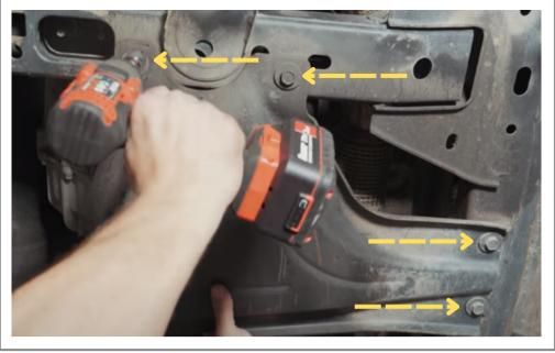
IF vehicle is equipped with skid plates remove the four 15mm bolts and remove the factory skid plate.
