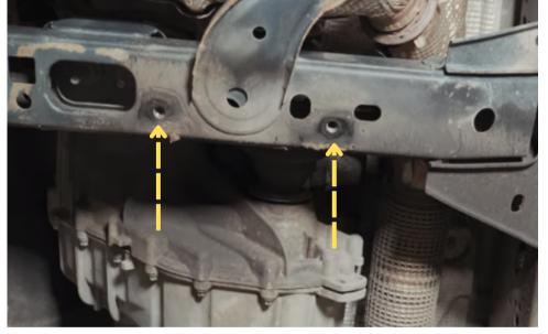
Install two 6mm allen bolts and washers half way.
