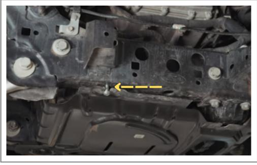
Install **one** 6mm allen bolt with washer for the rear of the skid plate to slide onto.
