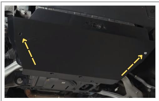
Step 6 Install **two** 6mm allen bolts with washers at the front of the skid plate.
