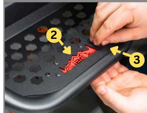
**Step 9:** Prepare the IAG Logo Plate and four provided 2.5mm Allen Bolts. Align the Logo Plate and install Bolts.
