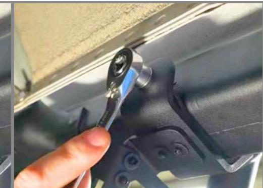
**Step 8:** Using a 10mm Wrench, tighten the Jam Nuts until snug.
