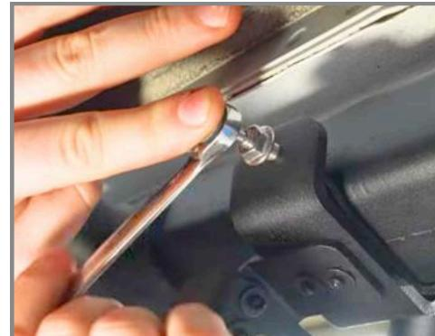
**Step 7:** Using a 3mm Allen Wrench, tighten the Mounting Studs until snug against the Rock Rail.
