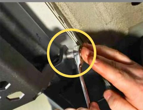
**Step 4:** Using a 10mm Wrench, tighten the Jam Nuts until snug.
