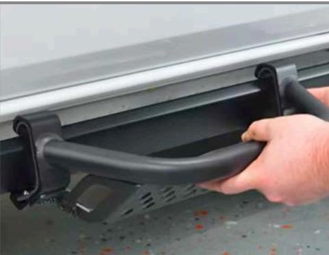
**Step 2:** Install the IAG Drop Step onto the front of the factory Rock Rail. Adjust step to desired position.
