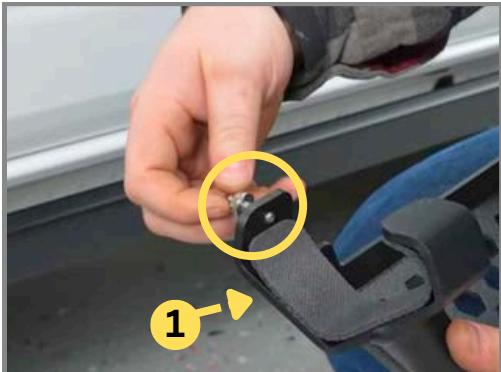
**Step 1:** Prepare the IAG Drop Step. Back out the mounting studs by hand until the end is flush with the bracket.
