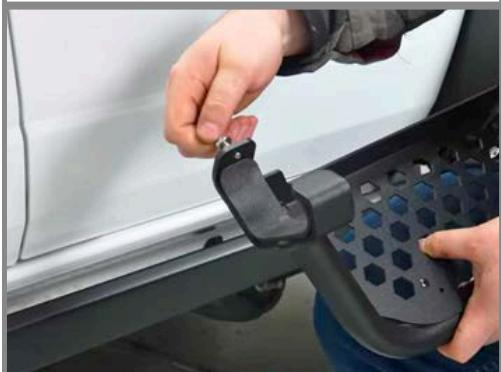
**Step 5:** Prepare the IAG Drop Step. Back out the mounting studs by hand until the end is flush with the bracket.
