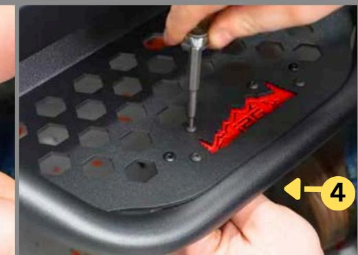
**Step 10:** Install provided 7mm nuts onto the Allen Bolts and tighten. Repeat for other side.
