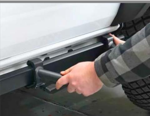
**Step 6:** Install the IAG Drop Step onto the rear of the factory Rock Rail. Adjust step to desired position.
