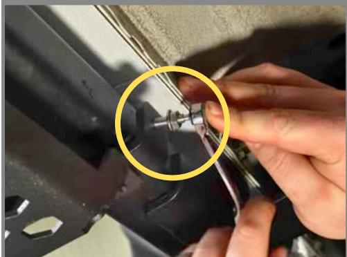
**Step 3:** Using a 3mm Allen Wrench, tighten the Mounting Studs until snug against the Rock Rail.
