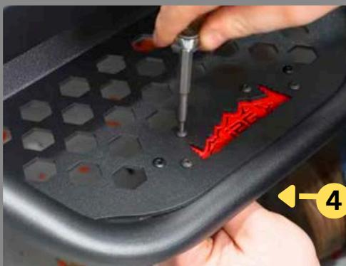
**Step 5:** Prepare the IAG Logo Plate and four provided 2.5mm Allen Bolts. Align the Logo Plate and install Bolts.
