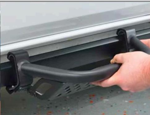
**Step 1:** Prepare the IAG Drop Step. Back out the mounting studs by hand until the end is flush with the bracket.
