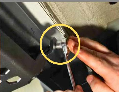
**Step 3:** Using a 3mm Allen Wrench, tighten the Mounting Studs until snug against the Rock Rail.
