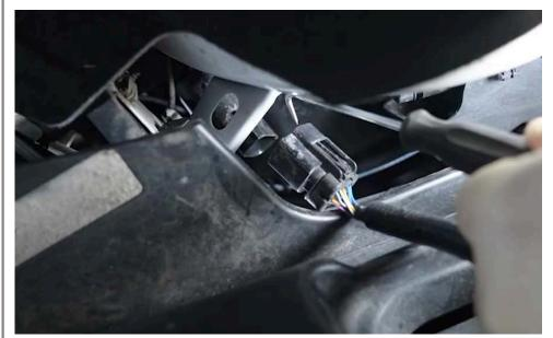
Disconnect the Bumper Harness inside the driver side fender.
