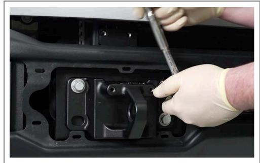
To adjust bumper alignment, loosen the six bumper bolts approximately half a turn.
