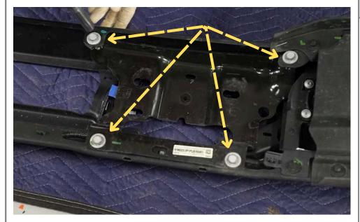
On the back of the bumper, remove the four 13mm bolts from the passenger side bumper plate.
