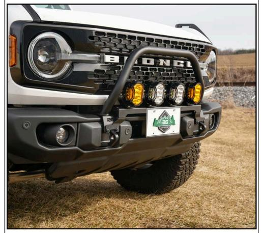
IAG Lower Light Mount Bar For 2021+ Bronco Capable Bumper IAG Lower Light Mount Bar for 21+ Bronco Capable Bumper Part Number: IAG-BDY-F1410
