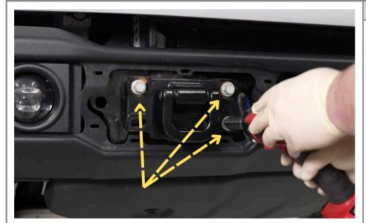
Remove the six 15mm bumper bolts from the recovery points.
