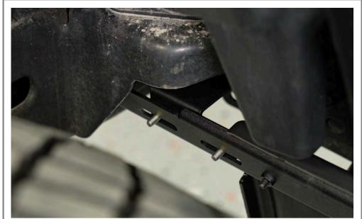
Install the Mud Flap Slider onto the studs of the Lower Bracket
