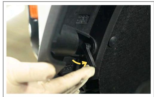
Remove the rear fender flare from the drivers side.
