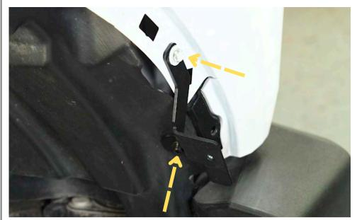
Install the bracket onto the fender.
