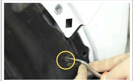
Remove shown push clip from fender liner and fold fender liner aside.
