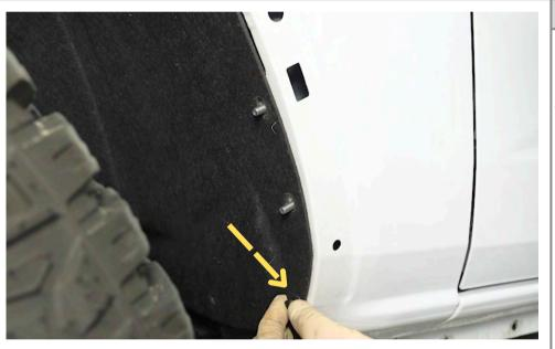
**Step 4** Reinstall the fender liner, reuse one of the factory push clips as shown.
