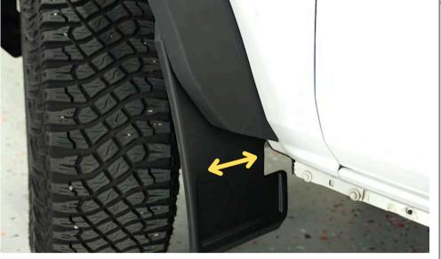
Adjust Mud Flap to align with fender flare, then tighten the mudflap hardware.
