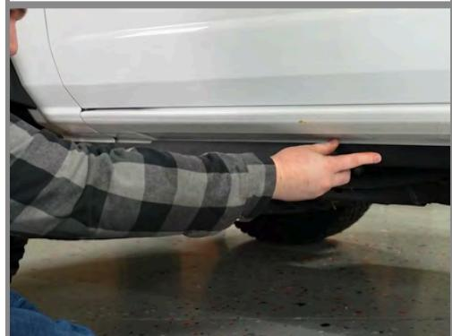
**Step 3:** Install the Pinch Weld Cover onto the front of the Pinch Weld.
