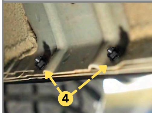
**Step 9:** Install and tighten two provided 10mm nuts onto the rear studs. (10Nm)
