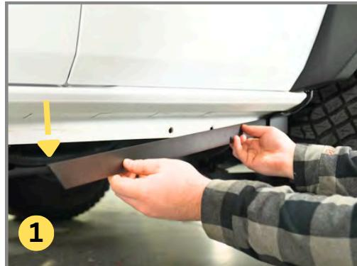
**Step 7:** Locate the Rear Left Pinch Weld Cover. Note the slanted cut.
