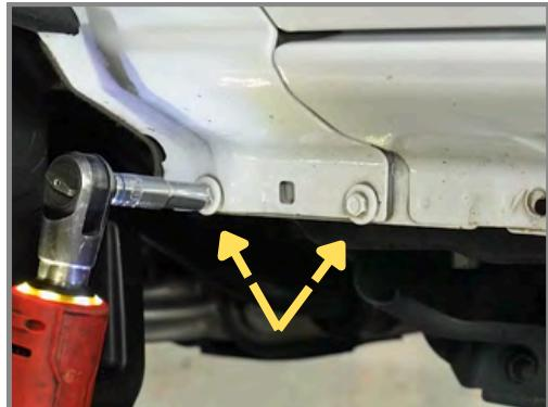
**Step 1:** Remove the two factory 10mm bolts from the bottom of the Driver Side Front Fender.
