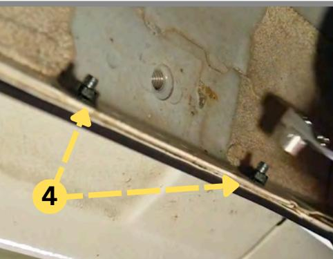
**Step 4:** Install and tighten two provided 10mm nuts onto the front studs. (10Nm)
