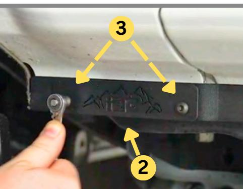
**Step 6:** Install the Logo Plate and two provided 4mm Allen Bolts into the Front Fender. (10Nm)
