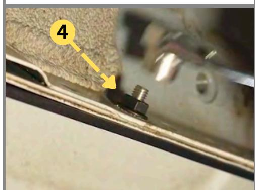
**Step 5:** Install and tighten provided 10mm nut onto the rear stud. (10Nm)
