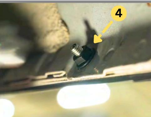
**Step 10:** Install and tighten provided 10mm nut onto the front stud. (10Nm)
