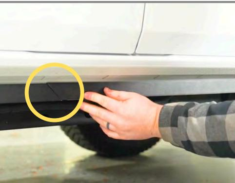
**Step 8:** Install the Pinch Weld Cover onto the rear of the Pinch Weld. Align with the Front Pinch Weld Cover.
