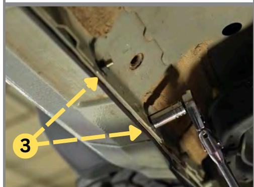
**Step 5:** Install and tighten two provided 10mm nuts onto the front studs. (10Nm)
