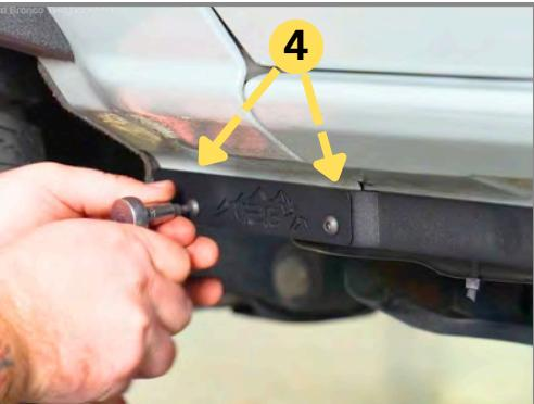
**Step 8:** Install the Logo Plate and two provided 4mm Allen Bolts into the Front Fender. (10Nm)
