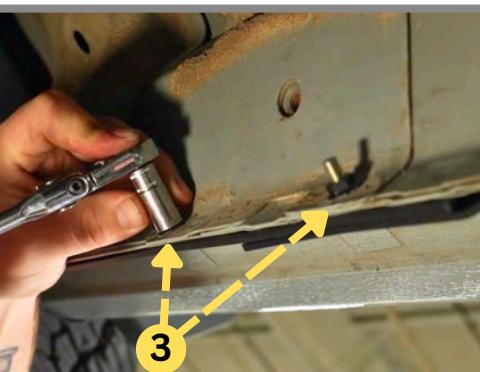
**Step 6:** Install and tighten two provided 10mm nuts onto the rear studs. (10Nm)
