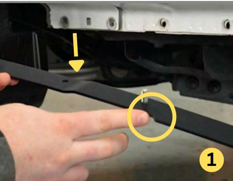
**Step 2:** Locate the Front Left Pinch Weld Cover. Note the upward facing notch, and the outward facing jogged bend.
