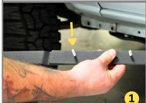
**Step 3:** Locate the Rear Left Pinch Weld Cover. Install the stud of the Front Cover through the hole of the Rear Cover.
