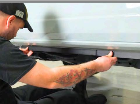
**Step 4:** Install the assembled Pinch Weld Covers onto the Pinch Weld.
