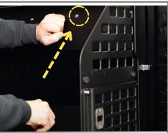
**Step 10/12:** Install a washer and nut to the **top** four studs.
