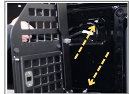
**Step 9/12:** Line up tailgate holes with studs.
