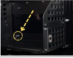
Step 11/12: Install a washer and nut to the bottom two studs.
