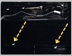
**Step 7/12:** Install each t-bolt to the inside of the slot and tighten. **Step 6/12:** Install the lower t-bolts with washer first and then a nut.
