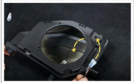
Prepare the new Speaker Pod and Speaker Wiring Harness. Route the wiring harness through the hole in the speaker pod as illustrated.
