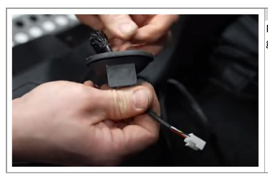
Step 12 Pass wiring harness through grommet
