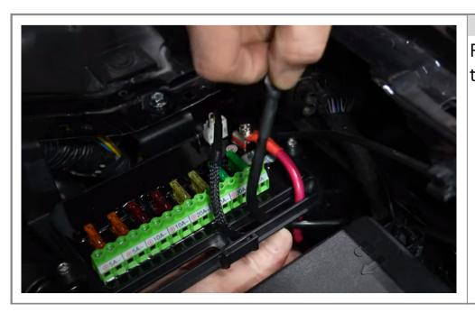
Step 36 Route negative wire up through channel in fuse box
