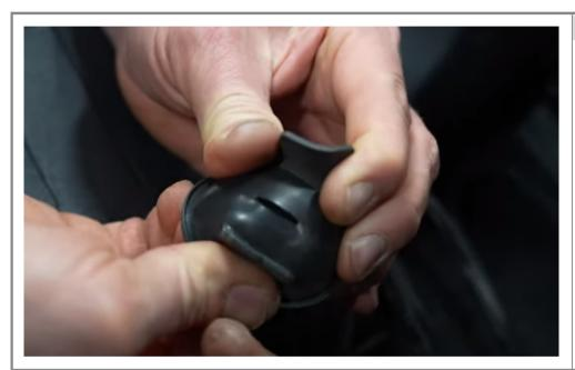
Step 11 Cut slit into grommet for wire to pass through using a razor blade
