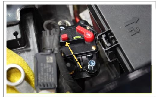
Step 25 Open the circuit breaker by pressing on the red button
