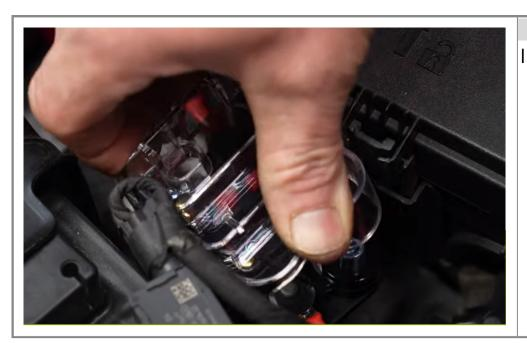
Step 49 Install circuit breaker cover
