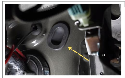
Step 10 Remove grommet to the left of brake pedal
