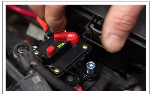
Step 48 Turn on circuit breaker by pushing red level closed
