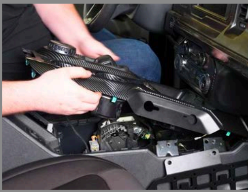
Step 4: Using a plastic pry tool, pry up on the center console trim and loosen. Complete removal is not necessary.
