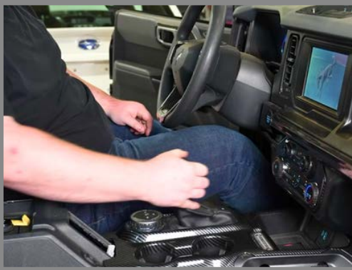
Step 3: Turn the key on with engine off. Apply the parking brake, and shift to neutral.
