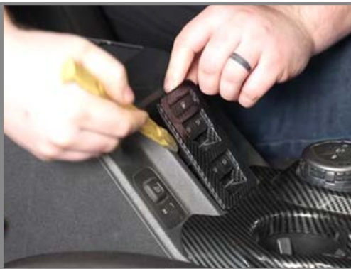
Step 1: Using a plastic pry tool, pry up and remove the Window Switch.
