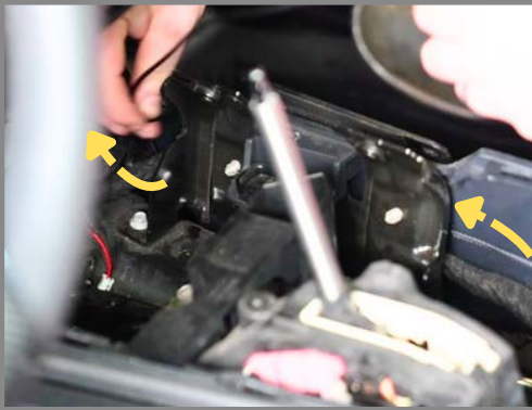
Step 6: Route the Adapter Harness along the factory wiring harness in the center console, towards the glove box.
