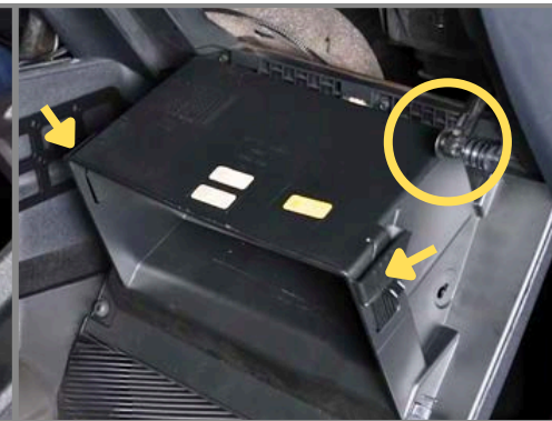
Step 8: Remove the Limiting Strap from the glove box. Depress the tabs on the side of the glove box and lower.
