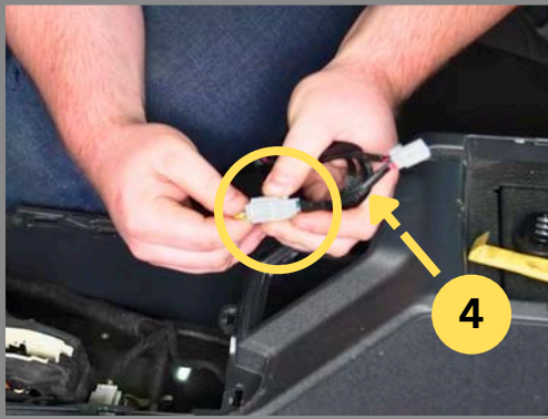
Step 5: Prepare the Adapter Harness. Plug the Adapter Harness into the factory wiring harness for the Window Switch.
