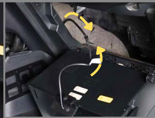
Step 10: Pull the remaining Adapter Harness through the glove box. Connect IAG Light to Adapter Harness.
