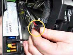
**Step 10:** Connect the Adapter Harness to the Fuse Adapter.
