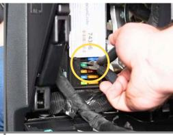
**Step 8:** Locate the 30 Amp fuse in the Driver side Fuse Box. Remove the fuse.
