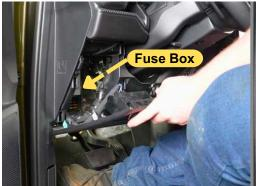
**Step 7:** Using a plastic pry tool, remove the trim from below the steering wheel, gaining access to the Fuse Box.
