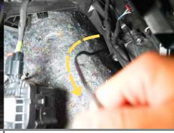
**Step 6:** Locate the Adapter Harness in the driver side foot well.
