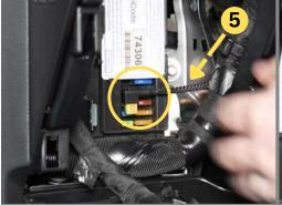
**Step 9:** Prepare the Fuse Adapter. Install the 30 Amp fuse into the Adapter. Install the Adapter into the Fuse Box.
