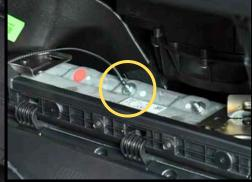
**Step 4:** Install the Spade Terminal of the Adapter Harness to the 10mm nut behind the Glove Box as shown.
