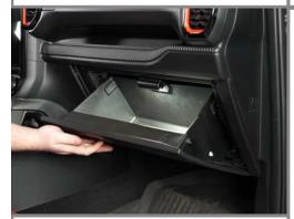
**Step 11:** Reinstall Glove Box and Trim. Use provided Zip ties to secure Harness away from steering column.
