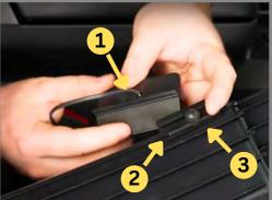
**Step 2:** Prepare the IAG Light and Bracket. Install the Bracket onto the back of the glove box and slide the Light into the Bracket. Secure with thumb screw.
