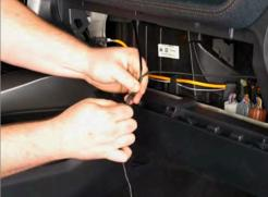
**Step 10:** Connect the Adapter Harness to the Glove Box Light.
