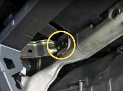
**Step 3:** Locate the 8mm Bolt on the Dash Support Bar, behind the glove box. Loosen the bolt, but do not remove.
