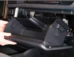
**Step 2:** Remove the Glove Box from the vehicle.
