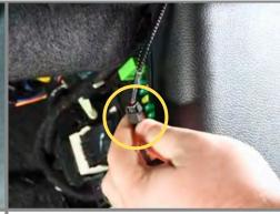
**Step 8:** Route the Adapter Harness towards the fuse box and connect the fuse adapter. Tuck harness behind trim.
