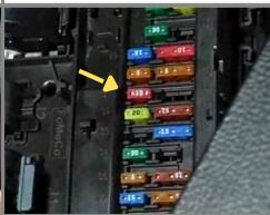
**Step 6:** Locate the 10 amp micro fuse about halfway up the fuse box. Remove the fuse.
