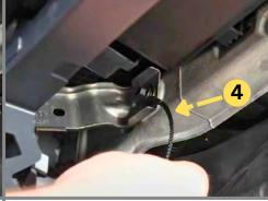
**Step 4:** Prepare the Adapter Harness. Slide the spade connector underneath the bolt and tighten.
