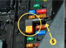
**Step 7:** Prepare the Fuse Adapter. Install the 10 Amp fuse into the Adapter. Install the Adapter into the Fuse Box.
