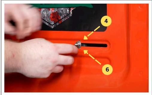
Prepare the M6 T Studs with Washers and Nuts.
