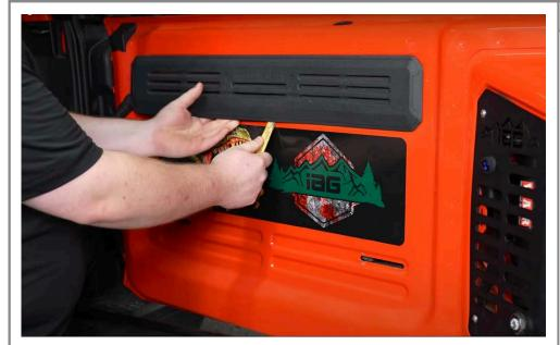
Using a plastic trim pry tool, remove the interior trim panel from the tailgate.
