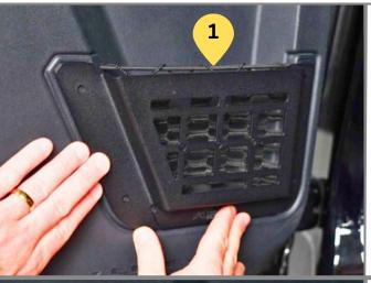
Step 1: Align the Left Door Bin with the driver side Rear Door Pocket.
