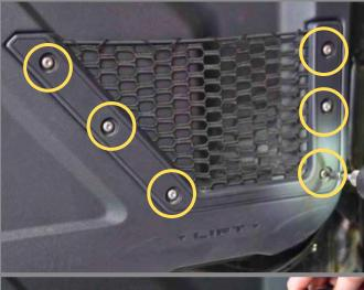
Step 1: Remove the six Torx 30 Bolts from the factory Door Pocket.
