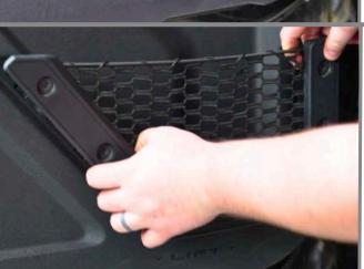
Step 2: Remove the factory Door Pocket Trim and Net.
