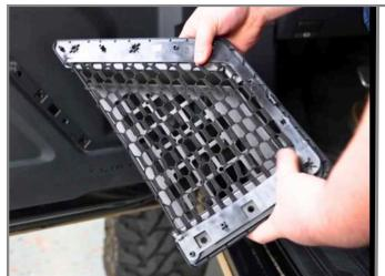
Step 4: Install the factory Pocket Net on the backside of the IAG Door Bin.
