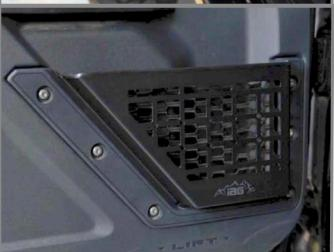
Step 5: Install the IAG Door Bin onto the vehicle. Reinstall the six factory bolts and tighten.
