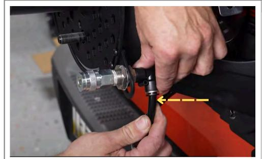
Install the other end of the soft 19" air line from the passenger side of the tank to the air tap fitting.
