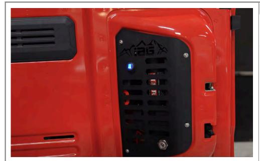
Turn the compressor on to fill the tank. Compressor turns off when tank is full.
