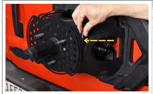
The soft 19" air line can route to the top or bottom depending on air tap location.
