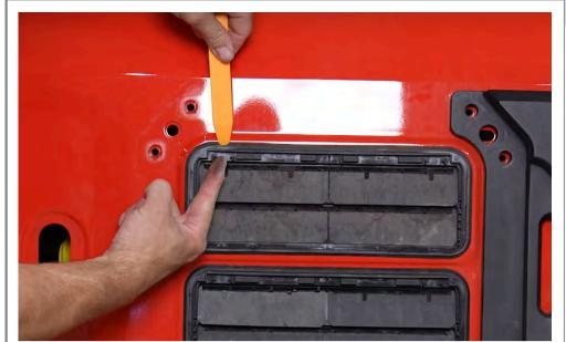
With a trim panel pry tool push down on the three clip locations to remove the upper air flap plate.
