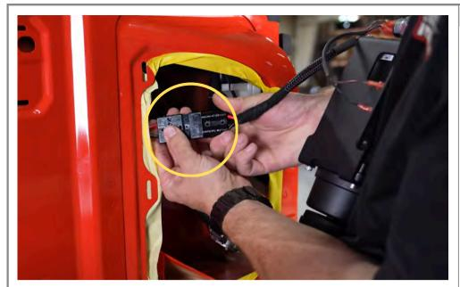
Install the compressor harness to the relay harness from step 52.
